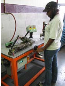
Illustration 10 Leak Decay Test Fixture
