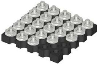
Illustration 6 Braze Fixtures to Hold parts in Location During Brazing
