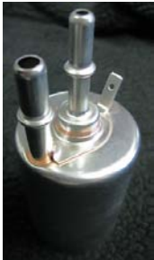
Figure 6 Fuel Filter Housing
