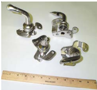
Figure 2 Stainless Steel Automotive Fitting – Copper Brazed
