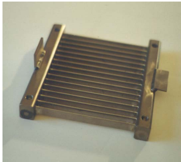
Figure 2 Stainless & Inconel Heat Exchanger GTAW & Nickel brazed
