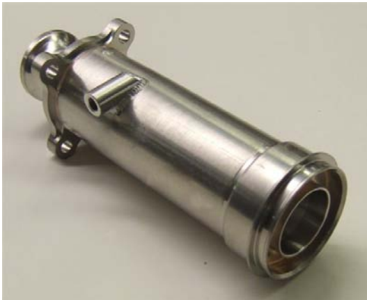
Figure 1 Aircraft Bleed Air Fabrication GTAW Welded and Hydrogen Brazed
