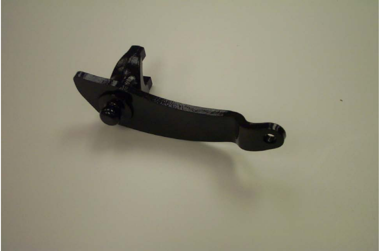
Figure 3 Braking Lever: assembled brazed and heat treated
