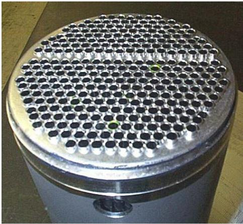
**Nickel brazed tube bundle heat exchanger**
