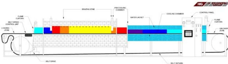
A straight through, continuous belt furnace avoids many of the issues presented by the hump in the humpback furnace. However, a straight through furnace is not best suited for brazing stainless steels because of the difficulty of controlling the furnace dew point. With a straight through furnace the belt rides on a horizontal surface throughout the furnace. Product stability and height issues are minimized along with the added maintenance that is seen in the humpback furnace
