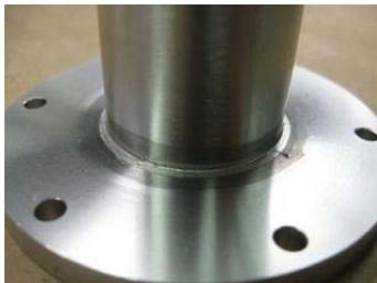
Nickel Brazed Stainless Steel Detector Tube
