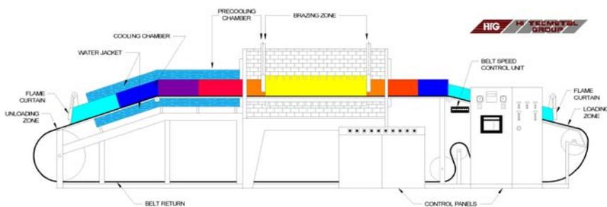
The humpback furnace affords the producer the ability to braze larger volumes of product with equivalent quality, higher production rates, and higher thermal efficiency **than the vacuum furnace**.
